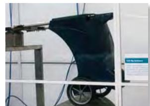
Skipper Trolley being Rolling Road tested.
