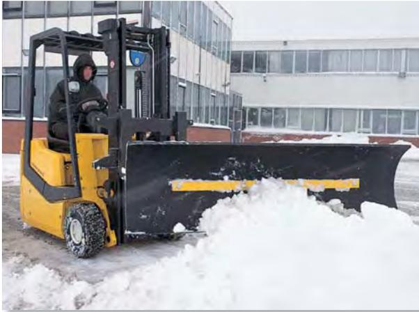
Your own forklift truck can soon be converted into a powerful and effective snow removal machine. The Glasdon Snowdozer is a unique, easy to fit attachment. Simply slide over the forklift truck forks and tighten fixings by hand to secure.
